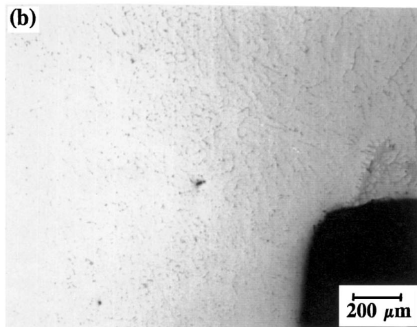
Figure 13 Optical micrographs taken from the region where the base section joins the biscuit section for 7050 alloy billets with a middle section thickness of 20 mm, manufactured by (a) gravity casting and (b) indirect squeeze casting.
